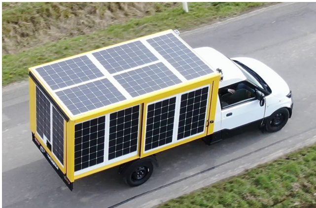
FIGURE 2 | Rear side flat PV modules visible on the prototype along with the irradiance sensor located near the bottom part (highlighted red) kg, with the weight of added PV and measurement systems being 320 kg. The weights of the individual components are noted in Table 2. For a similar commercial system, using the specific weight of flexible PV modules of 2.2 \text{ kg/m}^2 [4] and the balance-of-system (MPPTs, DC-DC converters, wiring, and mounting structures) of 10 kg, the total weight could be approximately 35 kg (without the buffer battery architecture).
